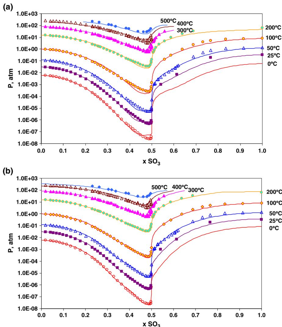
Fig. 6. Calculated and experimental vapor–liquid equilibria in the sulfuric acid/oleum system as a function of the mole fraction of  $\text{SO}_3$  at various temperatures from 0 to 500 °C. The results are obtained using (a) the  $\text{H}^+$  ion approach and (b) the  $\text{H}_3\text{O}^+$  ion approach (see text). Literature data are taken from Gmitro and Vermeulen [29], Brand and Rutherford [30], Schrage [31], and Giazitzoglou and Wuster [32].
