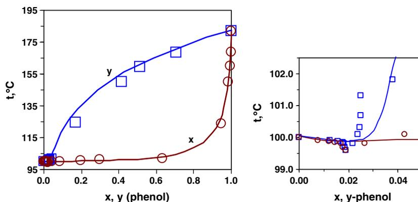
Fig. 1. Calculated and experimental VLE results for the phenol+H<sub>2</sub>O system at 1 atm. The symbols represent the data of Brusset and Gaynes [20].
