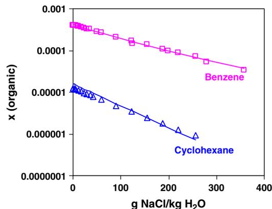
Fig. 4. Calculated and experimental solubilities of benzene and cyclohexane in aqueous NaCl solutions as a function of NaCl concentration (in g salt/kg H<sub>2</sub>O) at 25 °C. The symbols denote the data of Shaw [28] (benzene) and Xie et al. [27] (cyclohexane).
