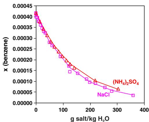
Fig. 3. Calculated and experimental solubilities of benzene in aqueous (NH<sub>4</sub>)<sub>2</sub>SO<sub>4</sub> and NaCl solutions as a function of electrolyte concentration (in g salt/kg H<sub>2</sub>O) at 25 °C. The symbols denote the data of Mackay and Shiu [26] and Xie et al. [27] (NH<sub>4</sub>)<sub>2</sub>SO<sub>4</sub>, and Shaw [28] (NaCl).
