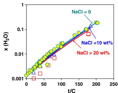
Fig. 5. Calculated and experimental solubilities of water in benzene as a function of temperature at the NaCl concentrations of 0%, 10%, and 20% (wt). The symbols denote the data of Shaw [28].
