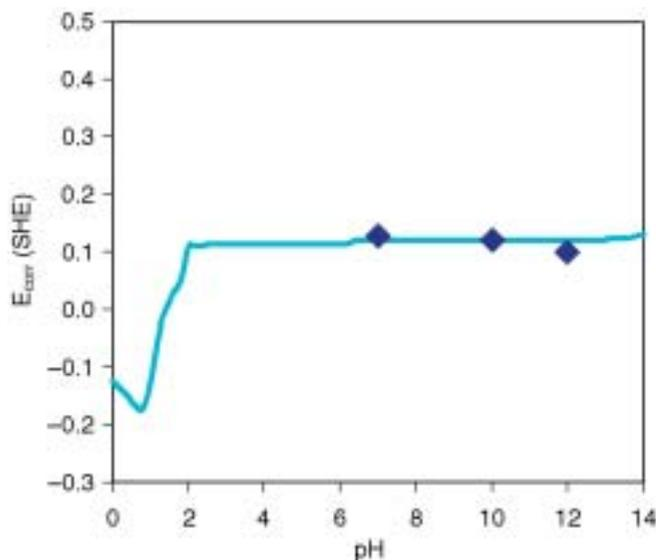
**FIGURE 8.** Experimental and calculated corrosion potentials of Type 316L SS in 0.5 m sodium sulfate ( $\text{Na}_2\text{SO}_4$ ) solutions with 0.32 ppm  $\text{O}_2$  as a function of pH (RCE, 1,000 rpm).
