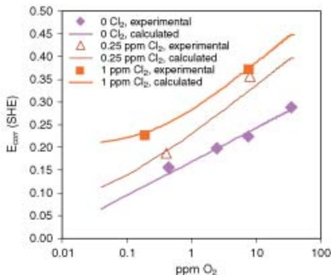
**FIGURE 6.** Experimental and calculated corrosion potentials of Type 316L SS in artificial seawater (RCE, 1,000 rpm) as a function of oxygen concentration for three concentrations of dissolved chlorine (i.e., 0, 0.25, and 1 ppm  $Cl_2$ ).
