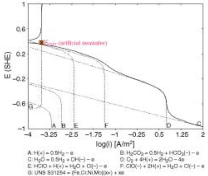
**FIGURE 17.** Calculated current density vs potential relationship for Alloy 254SMO SS in chlorinated seawater containing 7.62 ppm  $O_2$  and 1 ppm  $Cl_2$  at 25°C (rotation rate 1,000 rpm). The calculated corrosion potential is shown by the "x" symbol. The square shows the experimental corrosion potential in artificial seawater.
