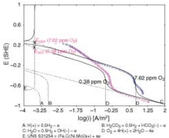
**FIGURE 22.** Comparison of calculated and experimental cathodic polarization curves for Alloy 254SMO SS in artificial seawater at 25°C in solutions containing 7.62 ppm or 0.38 ppm  $O_2$  (rotation rate 1,000 rpm).
