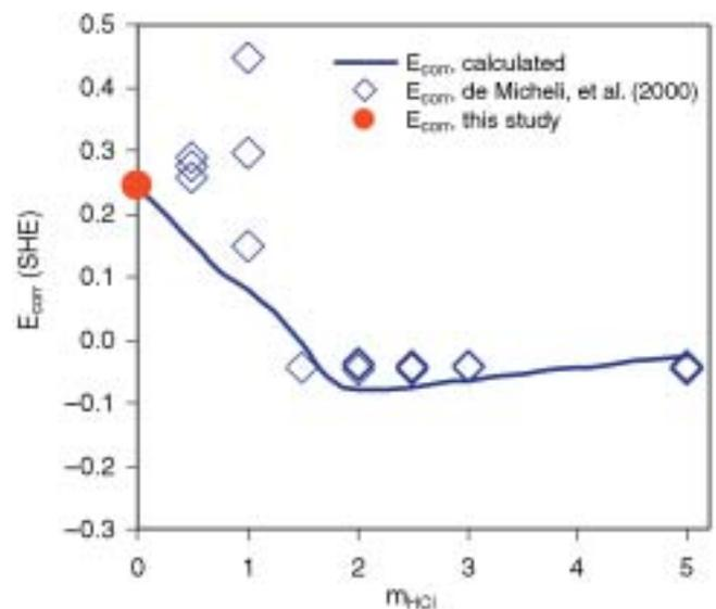
**FIGURE 10.** Effect of acidity on the corrosion potential of Alloy 254SMO SS in aerated solutions. The symbols denote the experimental data obtained in this study for neutral solutions and those of de Micheli, et al.,<sup>35</sup> for HCl solutions. The lines have been calculated from the model.
