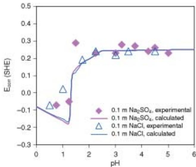
**FIGURE 9.** Effect of pH on the corrosion potential of Type 304 SS in aerated 0.1 m  $\text{Na}_2\text{SO}_4$  or sodium chloride ( $\text{NaCl}$ ) solutions. The symbols denote the experimental data of Leckie,<sup>34</sup> and the lines have been calculated from the model.
