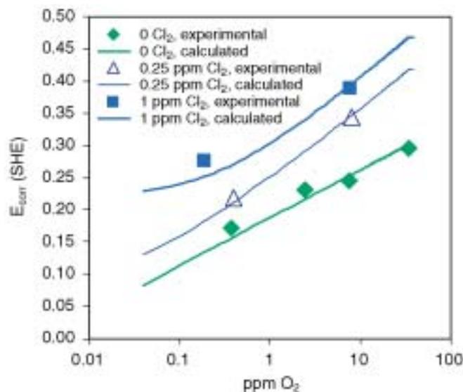
**FIGURE 7.** Experimental and calculated corrosion potentials of Alloy 254SMO SS in artificial seawater (RCE, 1,000 rpm) as a function of oxygen concentration for three concentrations of dissolved chlorine (i.e., 0, 0.25, and 1 ppm  $Cl_2$ ).
