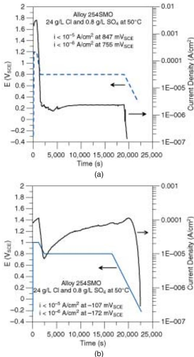
**FIGURE 2.** Effect of initiation potential on the repassivation potential of Alloy 254SMO. In case (a), no localized corrosion was initiated, just transpassive dissolution. The current was constant at the lower potential. For case (b), the current at 0.8  $V_{SCE}$  increased indicating localized corrosion.
