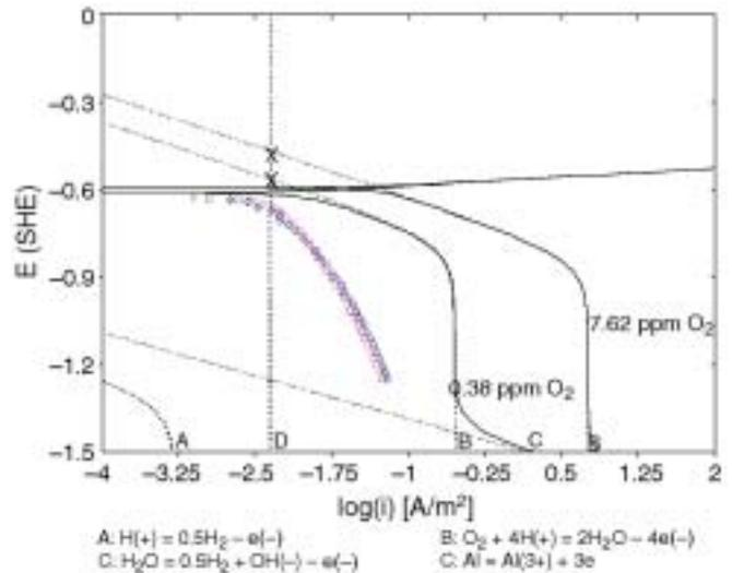
**FIGURE 23.** Comparison of calculated and experimental cathodic polarization curves for Al 1100 in artificial seawater at 25°C in solutions containing 7.62 ppm or 0.38 ppm  $O_2$  (rotation rate 1,000 rpm).
