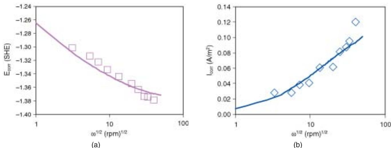
**FIGURE 11.** Calculated corrosion potential (left diagram) and corrosion rate (right diagram) for aluminum in a deaerated NaCl solution with pH = 9.02 as a function of the rotation speed of a rotating disk electrode. The symbols denote the experimental data of Craig and Scott.<sup>29</sup>
