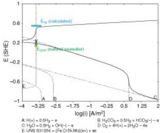
**FIGURE 18.** Calculated current density vs potential relationship for Alloy 254SMO SS in aerated seawater containing 5.6 ppm  $O_2$  at 35°C (rotation rate 1,000 rpm). The calculated corrosion potential is shown by the "x" symbol. The triangles show the experimental corrosion potential in natural seawater after 7 days and 14 days. The rectangle shows the calculated repassivation potential.
