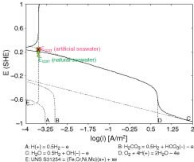
**FIGURE 16.** Calculated current density vs potential relationship for Alloy 254SMO SS in aerated seawater at 25°C (7.62 ppm of dissolved  $O_2$ , rotation rate 1,000 rpm). The calculated corrosion potential is shown by the "x" symbol. The square and triangles show the experimental corrosion potentials in artificial seawater (7.62 ppm  $O_2$ ) and natural seawater (6.8 ppm  $O_2$ ), respectively.
