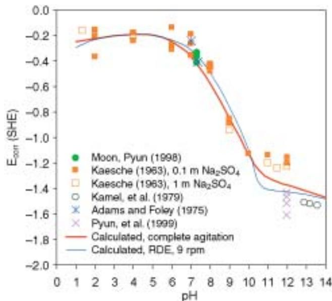
**FIGURE 13.** Corrosion potential of aluminum in aerated solutions that do not cause localized corrosion (i.e., aqueous  $\text{Na}_2\text{SO}_4$  or sodium hydroxide  $[\text{NaOH}]$ ) as a function of pH. The calculations have been made for two hydrodynamic conditions, i.e., for slowly flowing (RDE, 9 rpm) and completely agitated solutions. Experimental data was obtained elsewhere.<sup>28,58-61</sup>
