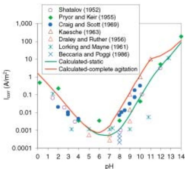
**FIGURE 12.** Calculated and experimental corrosion rates of aluminum as a function of pH. The calculated values were obtained for two extreme hydrodynamic conditions, i.e., static and completely agitated solutions. Experimental data were obtained from previous studies.<sup>28-29,53-57</sup>
