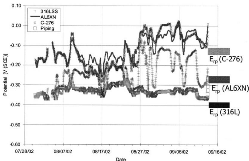
**6 Comparison of experimental corrosion potential data with predicted repassivation potentials for long term plant corrosion tests. Calculated repassivation potentials are depicted by rectangles. The height of the rectangles reflects the uncertainty of temperatures, which are assumed to vary from 95°C to 105°C**
