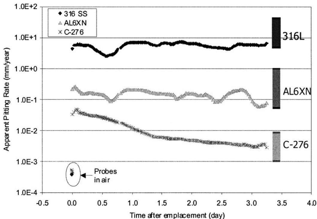
9 Comparison of experimental apparent pitting rates with calculated maximum rates of pit propagation for corrosion potentials obtained from short-term experiments (cf. Fig. 5). The vertical bars show the range of predicted pitting rates when the corrosion potential varies from  $-0.20$  V to  $-0.14$  V (vs SCE) and the temperature varies from  $95^{\circ}\text{C}$  to  $105^{\circ}\text{C}$
