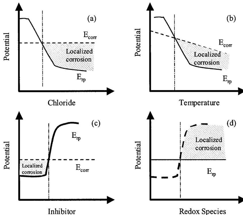
1 Schematic illustration of comparison of repassivation and corrosion potentials  $E_{rp}$  and  $E_{corr}$  for different environmental parameters. Shaded areas denote localised corrosion
