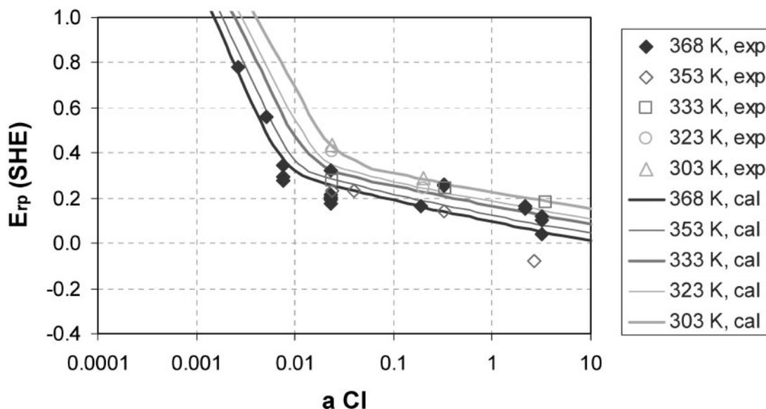
8 Effect of chloride activity (molality-based) and temperature on the repassivation potential of mill-annealed alloy 825. Experimental data are from Sridhar and Cragolino<sup>46</sup> and Anderko *et al.*<sup>19</sup>
