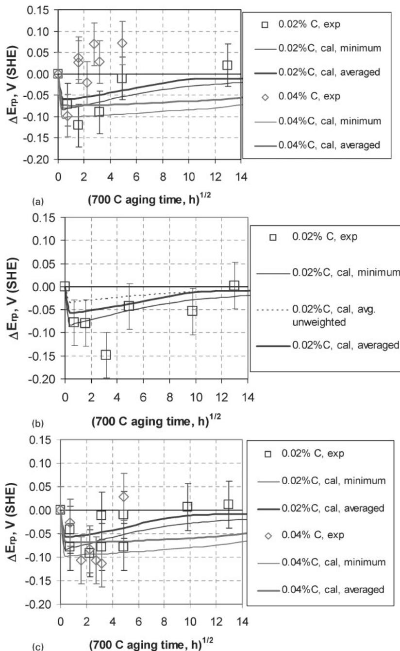
6 Predicted and experimental depression of the repassivation potential ( $\Delta E_{rp} = E_{rp} - E_{rp, \text{annealed}}$ ) of alloy 600 heat-treated at 700°C. The repassivation potential was obtained at 60°C in a 0.001, b 0.005 and c 0.04M NaCl solutions
