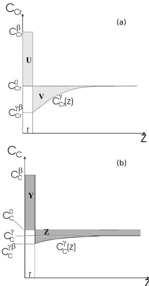
1 Scheme of grain boundary material balance calculations for Cr a and C b. Concentrations of Cr and C and denoted by  $C_{Cr}$  and  $C_C$  respectively. Superscripts 0,  $\beta$ ,  $\gamma$  and  $\gamma\beta$  denote concentrations in original alloy, carbide phase, bulk alloy and at alloy-carbide boundary respectively. The distance from the grain boundary is denoted by  $z$ , and  $r$  is dimension of grain boundary precipitate
