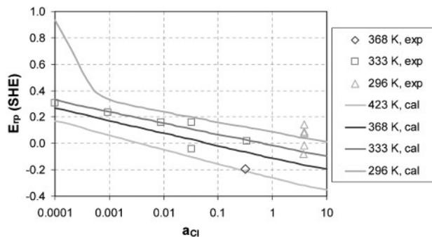
5 Effect of chloride activity (molality-based) and temperature on the repassivation potential of mill-annealed alloy 600
