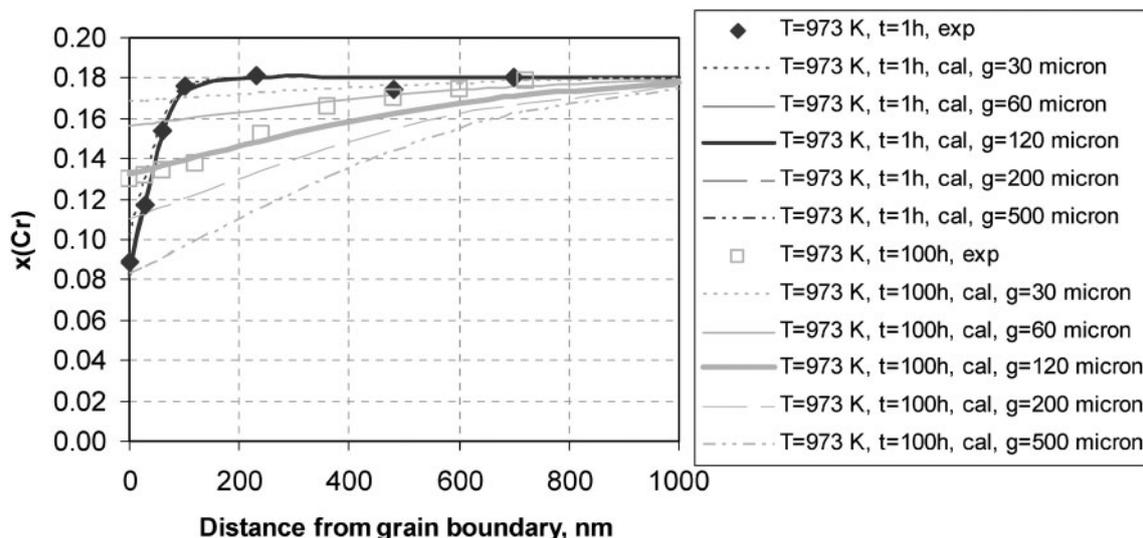
11 Effect of assumed grain size (ranging from 30 to 500  $\mu\text{m}$ ) on predicted Cr depletion profiles of alloy 600 heat treated at 973 K and 1 or 100 h. The experimental data of Was and Kruger<sup>10</sup> are shown for comparison
