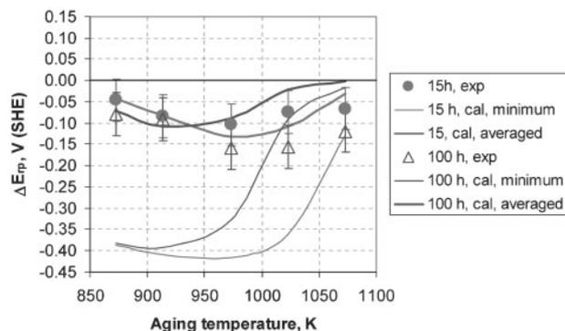
**10 Predicted and experimental depression of repassivation potential ( $\Delta E_{rp} = E_{rp} - E_{rp, \text{annealed}}$ ) of alloy 825 heat-treated at various temperatures. Repassivation potential was obtained at 95°C in 100 ppm (0.00282M)  $\text{Cl}^-$  solutions<sup>14</sup>**
