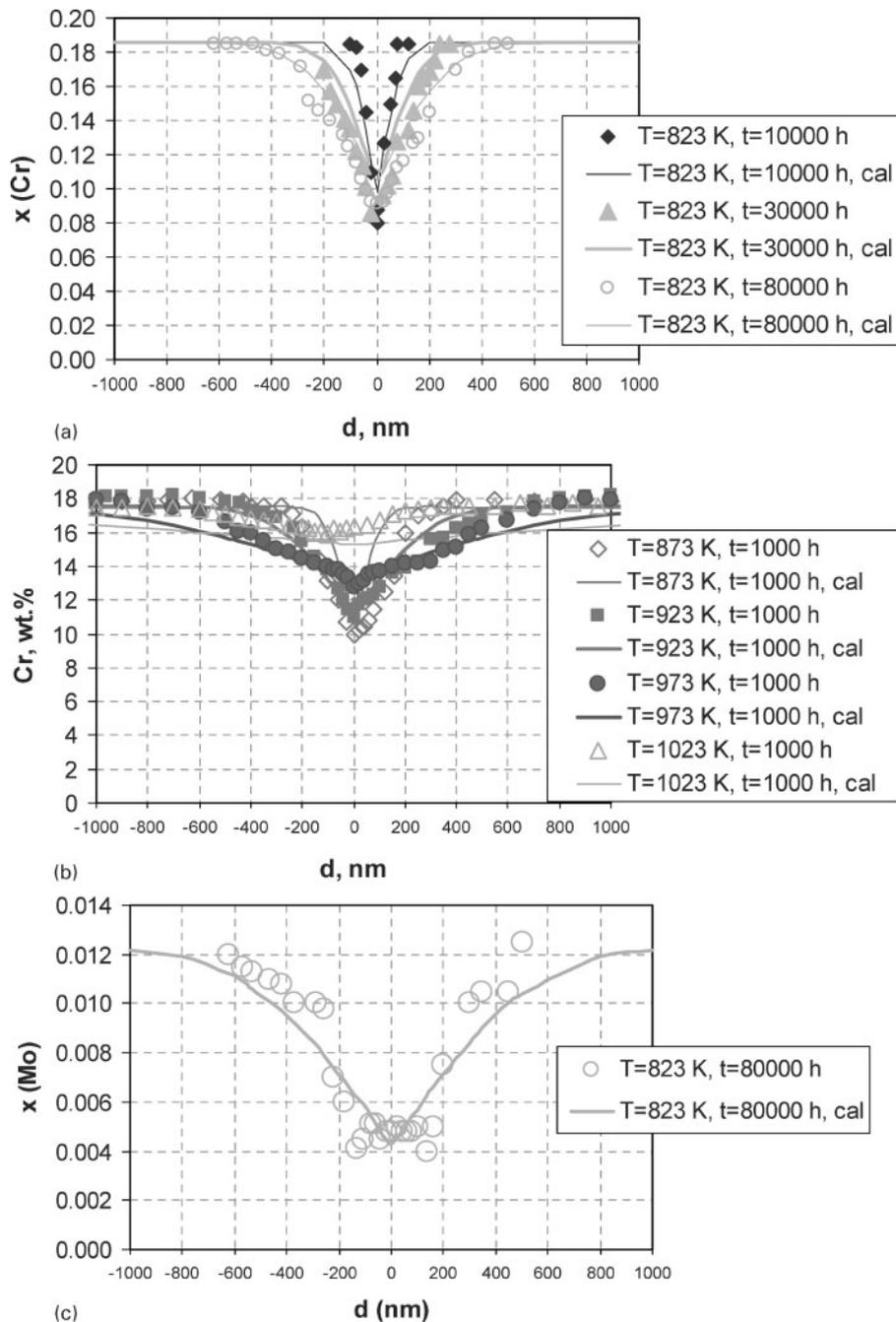
4 a, b Calculated and experimental chromium and c molybdenum depletion profiles for heat-treated type 316 stainless steel. The data are from Sahlouei et al.<sup>44</sup> (a, c) and Tekin et al.<sup>45</sup> (b)
