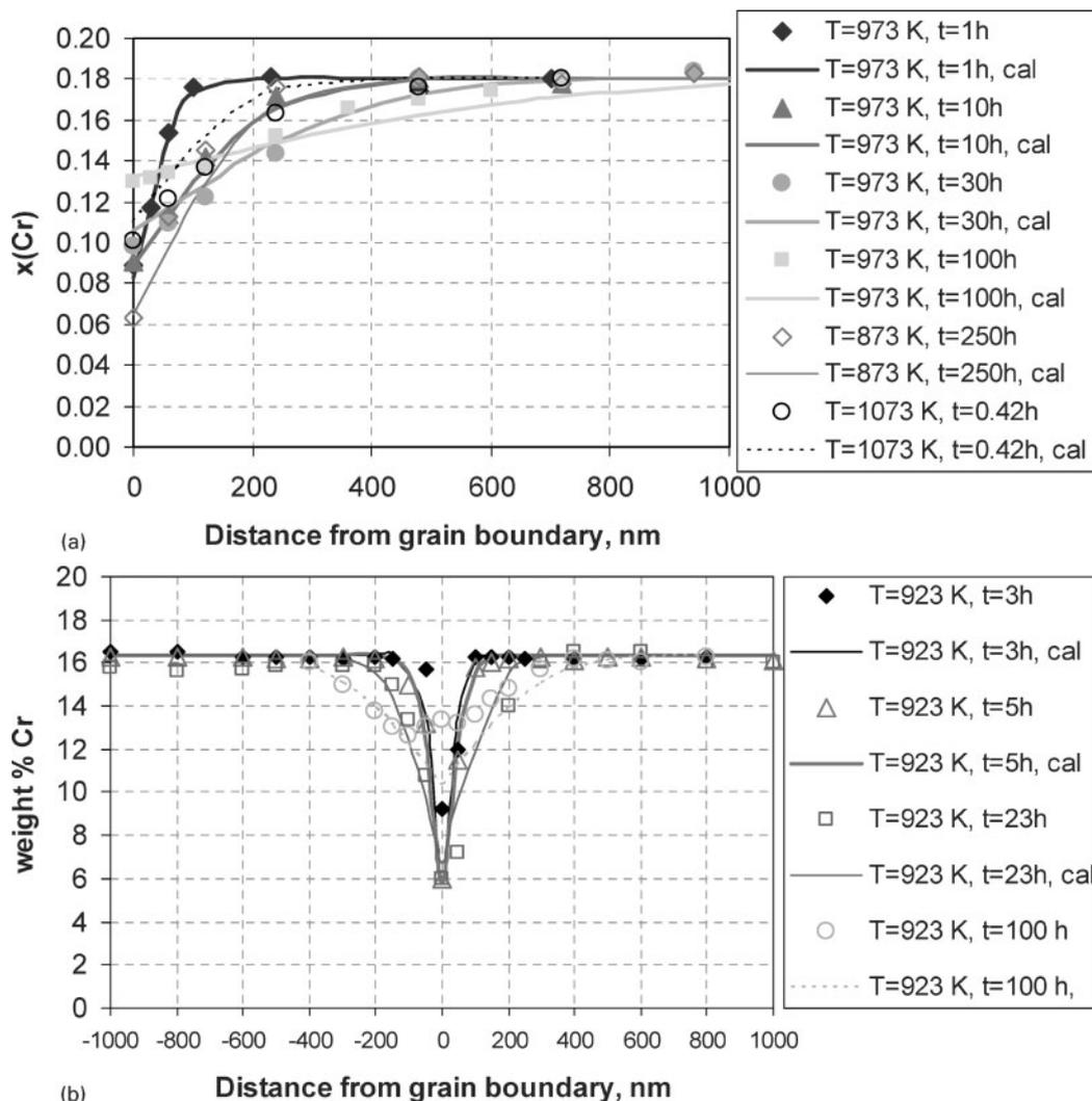
2 Calculated and experimental chromium depletion profiles of heat-treated alloy 600 for various aging temperatures and times. Experimental data are from Was and Kruger<sup>10</sup> a and Hall and Briant<sup>8</sup> b
