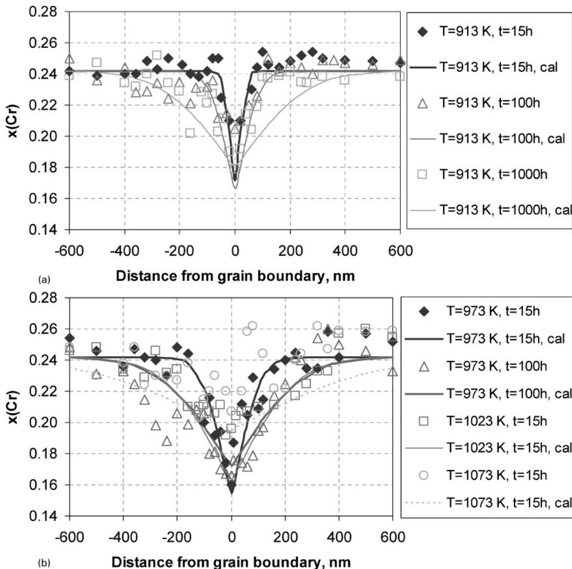
3 Calculated and experimental chromium depletion profiles for alloy 825 thermally aged at *a* 913 K and *b* 973–1073 K. Experimental data are from Pan *et al.*<sup>14</sup>
