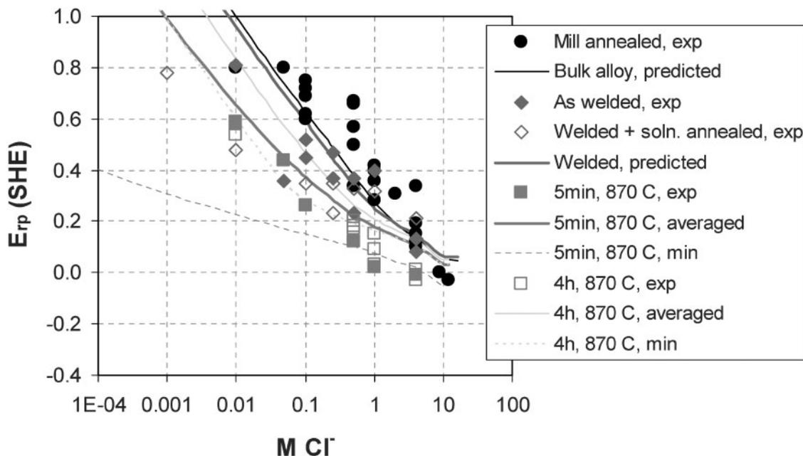
9 Predicted and experimental repassivation potential of alloy 22 as function of chloride concentration at 95°C in mill-annealed state, after welding and after welding followed by heat treatment at 870°C. Experimental data are from Dunn *et al.*<sup>15-17</sup>
