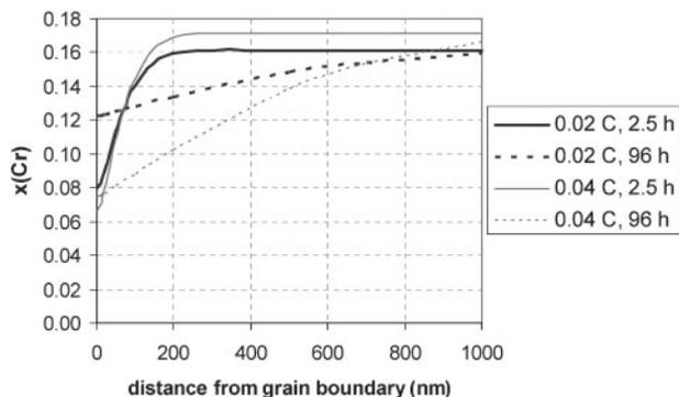
7 Predicted Cr depletion profiles for 0.02 and 0.04% C samples used for  $E_{rp}$  measurements<sup>18</sup> after heat treatment at 700°C
