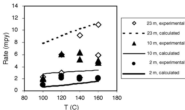
**FIGURE 7.** Corrosion rates of carbon steel in LiBr solutions at temperatures ranging from 100°C to 160°C and concentrations ranging from 2 m to 23 m. The experimental data were obtained by Tanno, et al.,<sup>3</sup> and the lines were obtained from the model.
