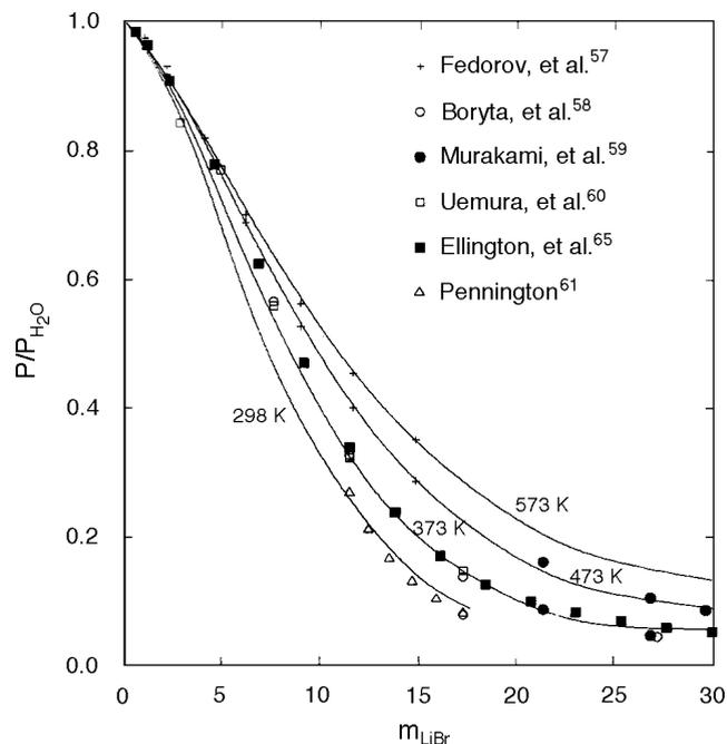
**FIGURE 1.** Saturated vapor pressures of aqueous LiBr solutions as a function of LiBr molality at various temperatures. The lines were obtained from the thermodynamic model and the symbols represent literature data.<sup>57-61,65</sup>
