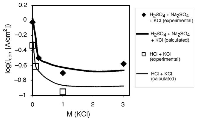
**FIGURE 3.** Effect of  $Cl^-$  concentration on the corrosion current for iron in  $H_2SO_4 + Na_2SO_4 + KCl$  and  $HCl + KCl$  solutions at  $25^\circ C$ . The lines were calculated from the model and the symbols represent literature data.<sup>18</sup>
