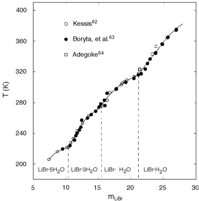
**FIGURE 2.** Solubility of various hydrates of solid phases in aqueous LiBr solutions. The lines were calculated from the thermodynamic model and the symbols represent literature data.<sup>62-64</sup>
