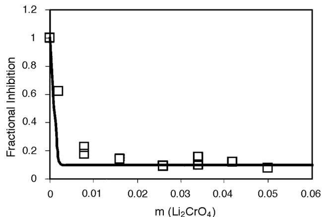
**FIGURE 12.** Effect of chromate ions on the corrosion rate in 13.52 m (54 wt%) LiBr + 0.18 m (0.2%) LiOH solution. The symbols denote literature data.<sup>48</sup>
