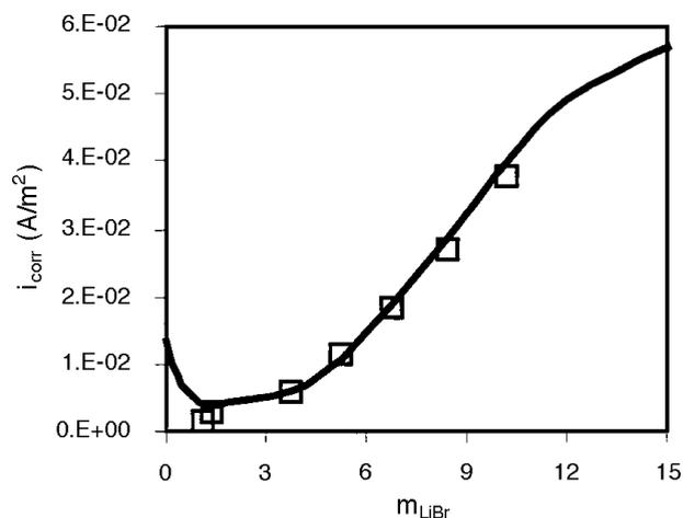
**FIGURE 6.** Corrosion rates for carbon steel in LiBr solutions of varying concentrations at 25°C. The lines were obtained from the model and the symbols denote literature data.<sup>2</sup>
