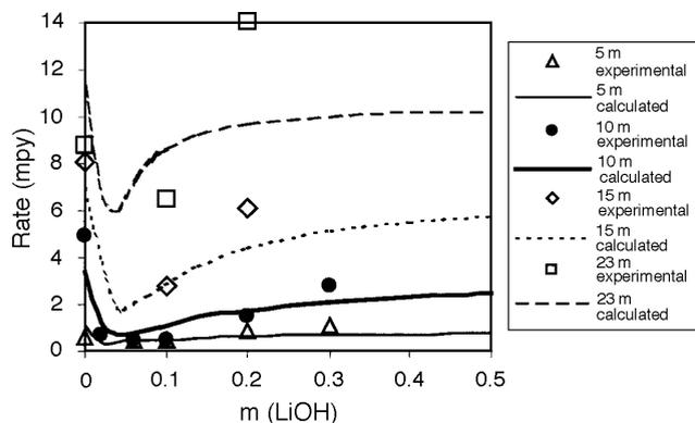
**FIGURE 8.** Corrosion rate as a function of LiOH molality for carbon steel at 160°C in LiBr solutions with various concentrations. The experimental data (symbols) were obtained by Tanno, et al.<sup>42</sup>
