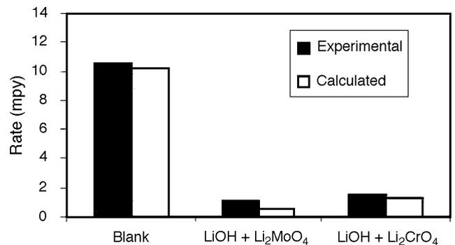
**FIGURE 11.** Corrosion rates of carbon steel in uninhibited and inhibited 20.47 m LiBr solution at 160°C. The molybdate-inhibited solution contained 0.24 m LiOH and 0.032 m  $\text{Li}_2\text{MoO}_4$ , and the chromate-inhibited solution contained 0.0066 m LiOH and 0.058 m  $\text{Li}_2\text{CrO}_4$ . The solid bars denote literature data.<sup>47</sup>
