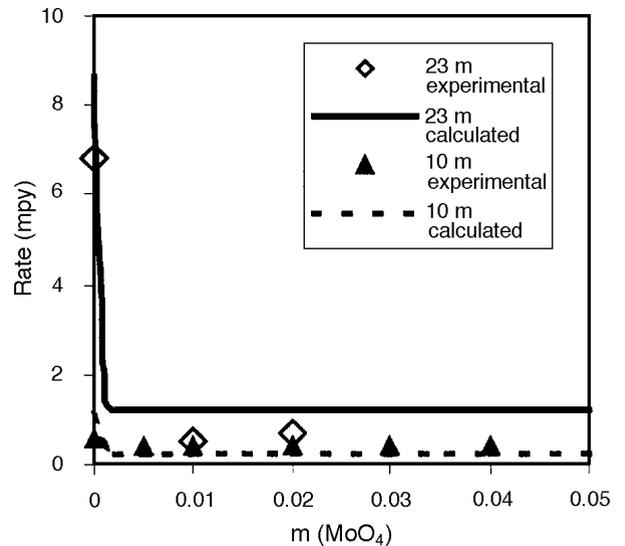
**FIGURE 10.** Effect of molybdate ions on corrosion rates of mild steel in solutions containing 0.1 m LiOH and various concentrations of LiBr. The symbols denote literature data.<sup>42</sup>
