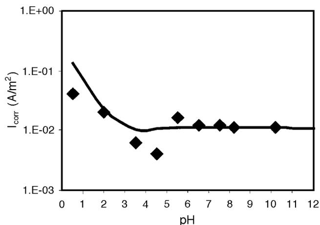
**FIGURE 5.**  $I_{\text{corr}}$  as a function of pH for carbon steel in a 4.6-M LiBr solution at 25°C. The line was calculated from the model and the symbols denote literature data.<sup>2</sup>
