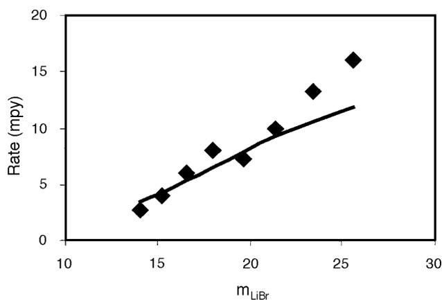
**FIGURE 9.** Corrosion rate of carbon steel in LiBr solutions of varying concentration at the normal boiling temperature (i.e., from 138.3°C at 14.07 m to 185.3°C at 25.63 m). Solutions were inhibited with 0.2 wt% LiOH. The line was calculated from the model and the symbols represent the literature data.<sup>43</sup>
