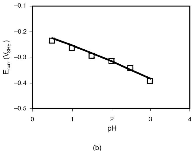
**FIGURE 4.**  $I_{corr}$  and  $E_{corr}$  of iron in a 1-M solution of HBr and KBr of varying acidity. The lines were obtained from the model and the symbols represent literature data.<sup>32</sup>
